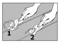
Trim the rod in 2 times : Directly after welding with a quartermoon knife (or Mozart knife) + the trimming guide. After the welding rod has cooled and without the trimming guide.
