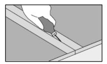
Apply the cold welding liquid by pressing the needle deeply into the seam **Ensure you apply enough liquid along the entire joint**. After 10 minutes the cold welding liquid on the masking tape should be dry and the masking tape is removed carefully backwards. **The seam can be walked on after 24 hours**.
