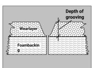
The grooving depth of seams must never be deeper than 2/3 of the thickness of the wearlayer.
