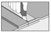
The sheets can be cold welded 24 hours after installation. Overlap the two sheets till the pattern match is achieved. The overlapping will be double cut in one step or two in case of thick flooring alongside a metal ruler. **The result shall be an extremely tight joint.**
