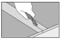
Fix a special masking tape, centered over the cut seam, then cut the masking tape with a rolling knife within the seam.
